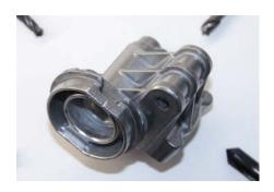
During deburring, the workpiece to be processed is, for example, mounted on the shuttle table and processed by brushing, grinding or milling. Even complex components, such as cylinder heads, hydraulic blocks or pump housings will be deburred, due to the multi-axle features of the deburring cells by gKteso. Aside from workpieces made from steel, grey cast iron, aluminum, brass or bronze, also plastic components produced through deep-drawing processes may be treated.
