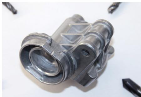
During deburring, the workpiece to be processed is, for example, picked up by the 2-jaw chuck and processed by brushing, grinding or milling. Even complex components, such as cylinder heads, hydraulic blocks or pump housings will be deburred, due to the multi-axle features of the deburring cells by gKteso. Aside from workpieces made from steel, grey cast iron, aluminum, brass or bronze, also plastic components produced through deep-drawing processes may be treated.
